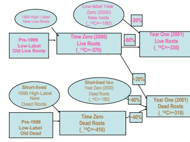
Figure 6. EBIS <sup>14</sup>C LABEL FLOW IN LIVE AND DEAD ROOTS—A simplified diagram of the flow of Carbon (and <sup>14</sup>C label) through Live and Dead Roots at highly-enriched sites from pre-1999 through 2001. Percentages transferred to create Year One pools are calculated estimates to balance changes in <sup>14</sup>C between all pools.
